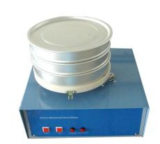
and oil plant, and determine insect density and judge grains grade. The sieves are made on aluminum. It can be used with our electric screen meter.
